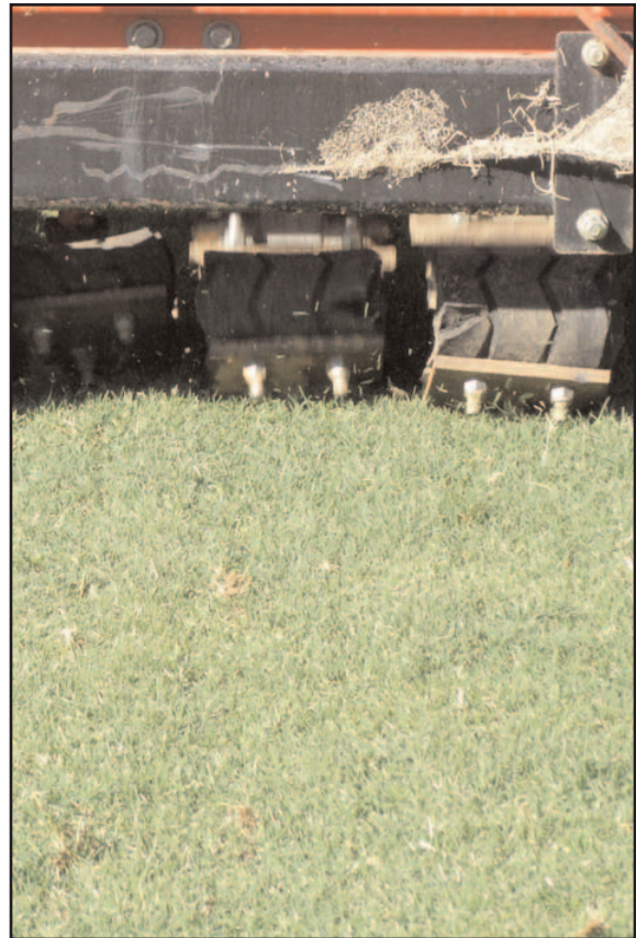
Device used to simulate traffic in turfgrass research
