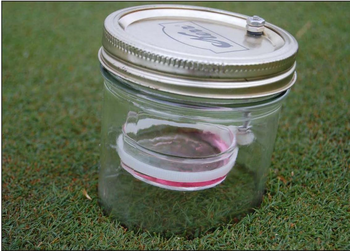
Fig. 1. Apparatus used for in-field ammonia volatilization estimates.
