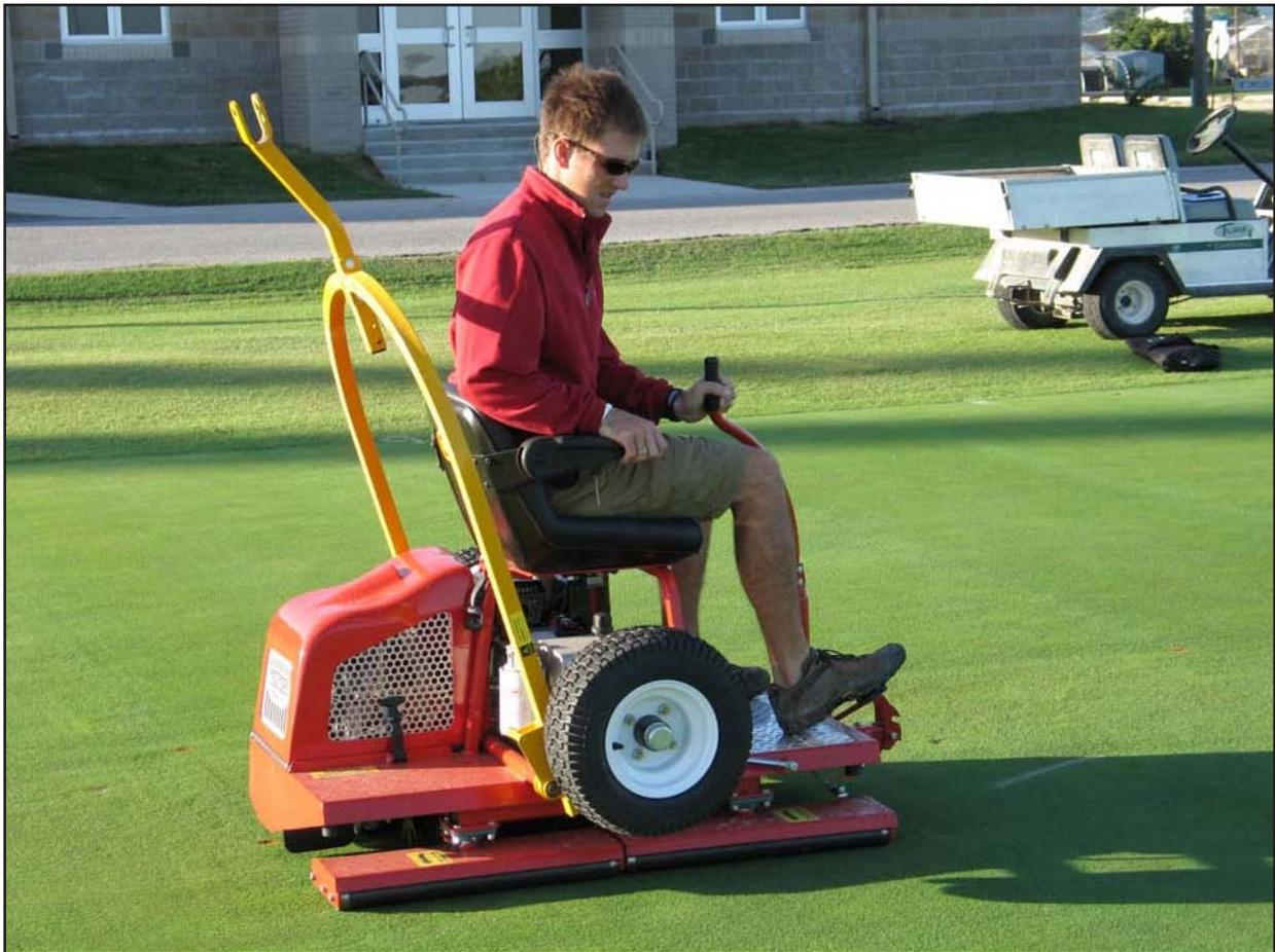
**Fig. 2. Tru-Turf roller that was used to apply treatments.**
