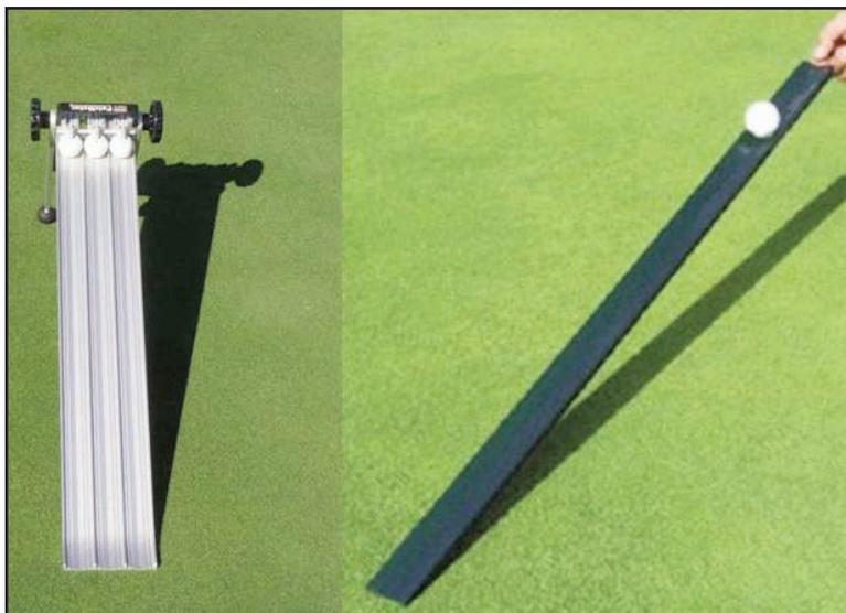
Devices used for measuring putting green speed. Pelzmeter (left) and Stimpmeter (right).
