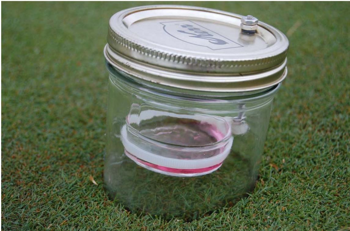
**Fig. 1. Apparatus used for in-field ammonia volatilization estimates.**
